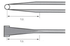
Trough change distance(T.D.)  $(T.D.) \ge Pipe diameter \times 25$
